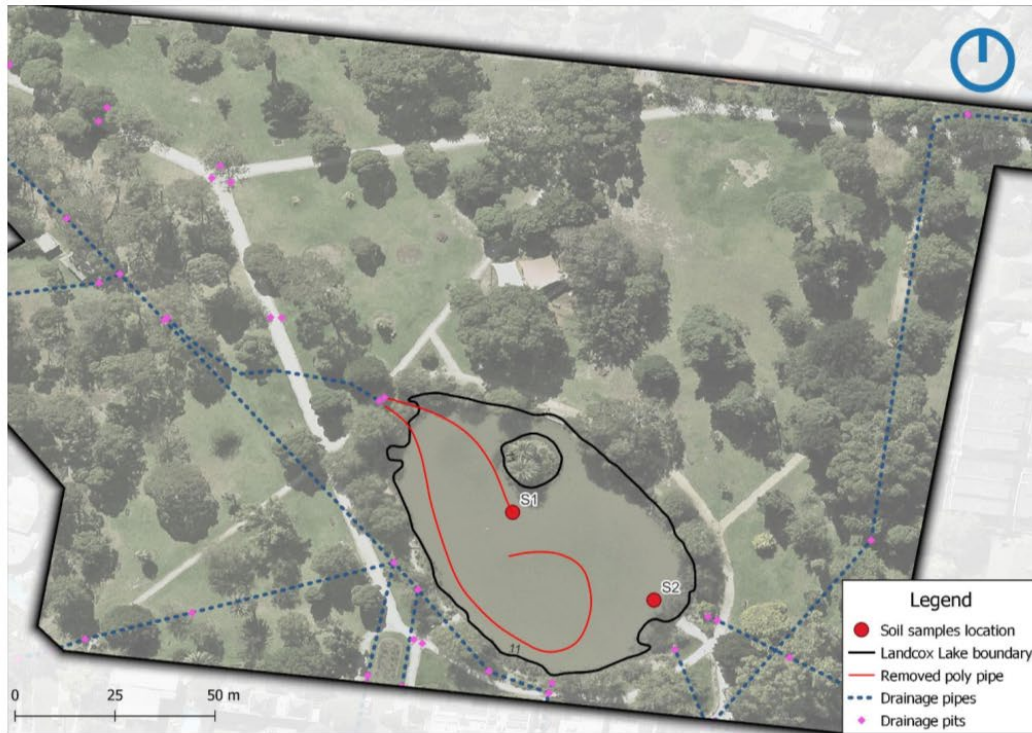
Figure 17. Soil sample location in the Landcox Park Lake context (Wave Consulting).
