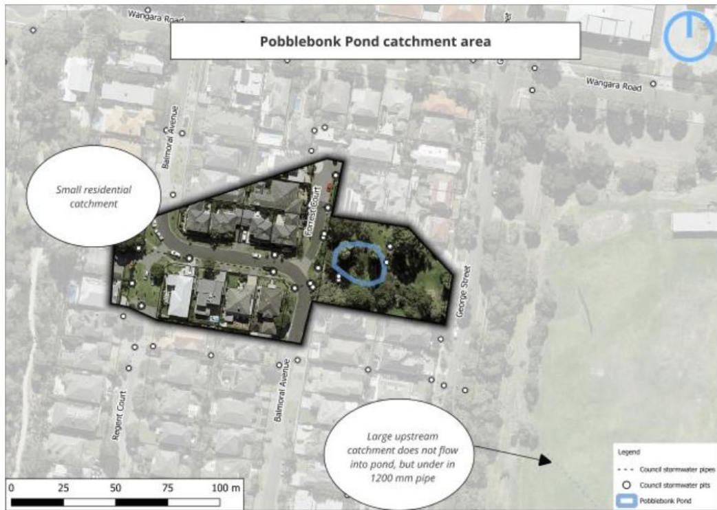
Figure 32. Catchments upstream of Pobblebonk Pond, with council drainage infrastructure (Wave Consulting).
