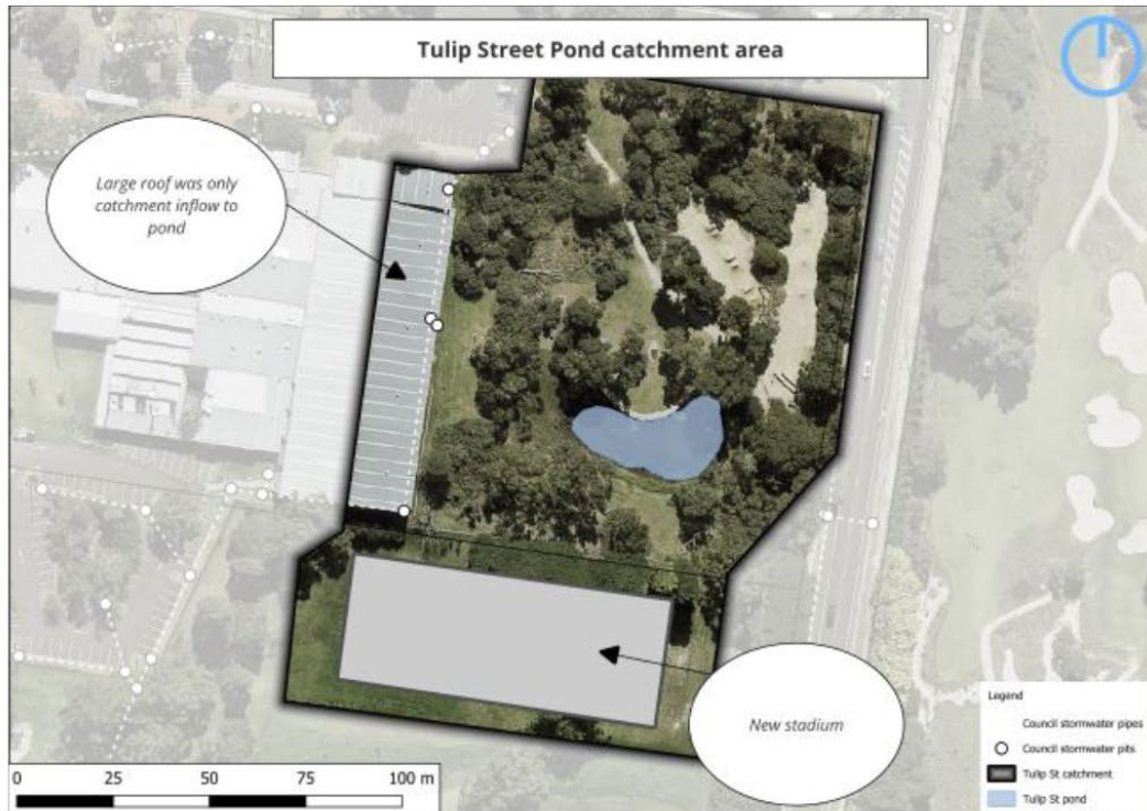
Figure 44. Catchments upstream of Tulip St Pond, with council drainage infrastructure (Wave Consulting).
