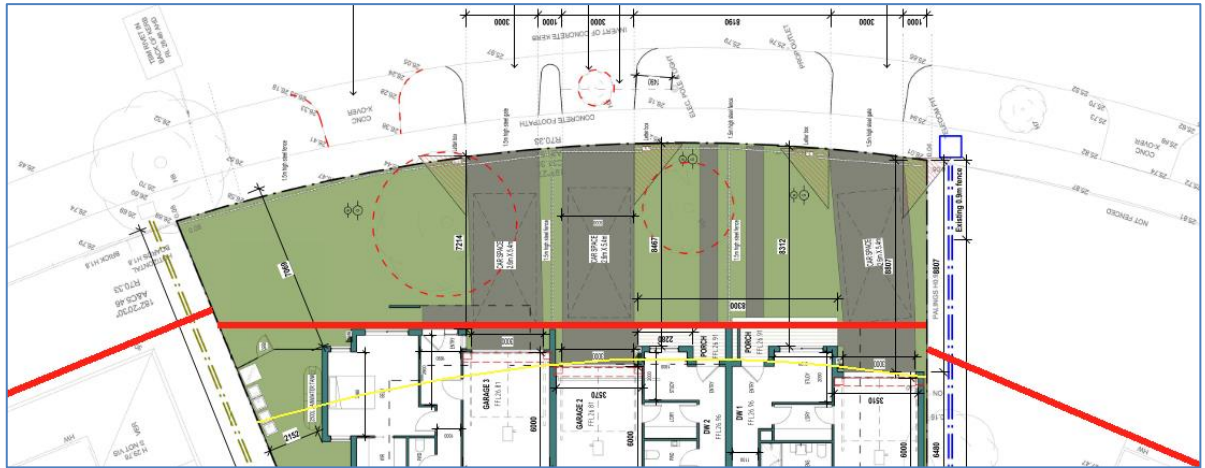
Image 2 Portion of ground floor plan with straight-line street setbacks of 3 and 5 Little Ave, and side setback of 12 Summit Ave extrapolated to the boundaries (red), and the 9-metre required setback to match the curved frontage (yellow)
